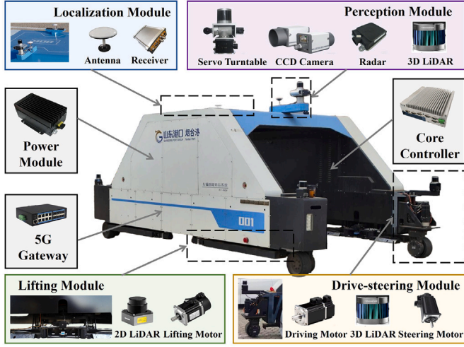
Fig. 6. Illustration of the AGV system physical platform.
