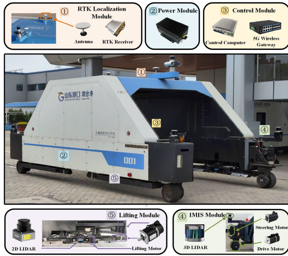
Fig. 1. Component structure of the AGV.
