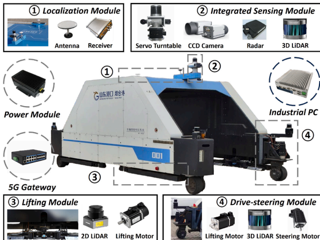
Fig. 10. Transfer robot hardware configuration and specifications.
