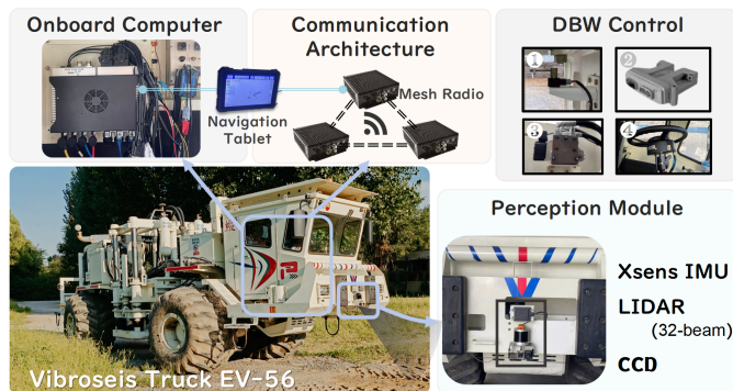
Fig. 12. Overview of the vibroseis truck platform and integrated hardware modules.
