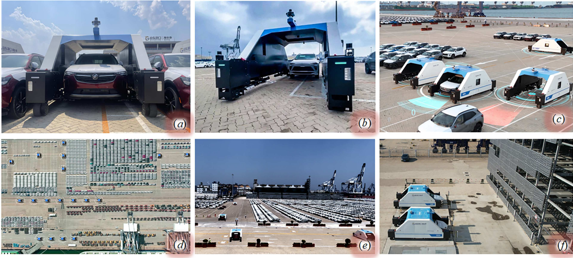
Figure 5 (Color online) Working process of finished vehicle transportation robots. (a) The transportation robots pick up finished vehicles; (b) the transportation robot places the finished vehicles in the parking space; (c) the transportation robot uses LiDAR to recognize the pose of finished vehicles; (d) the bird's eye view of the RO/RO logistics terminal; (e) the transportation robot moves to the stereo garage; (f) the transportation robot places the finished vehicle in the connection area of the stereo garage.
